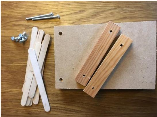
The dimensions of the base and the separation of the holes allows for 8 craft sticks which gives a simple octave. Six would work for Messy Church. One problem is that craft sticks, despite appearances, are not all the same thickness which means that when you screw down you may not securely clamp all of them. The thickness also affects the pitch, so you will see in my finished version that the lengths don't change regularly as you go up the octave.
